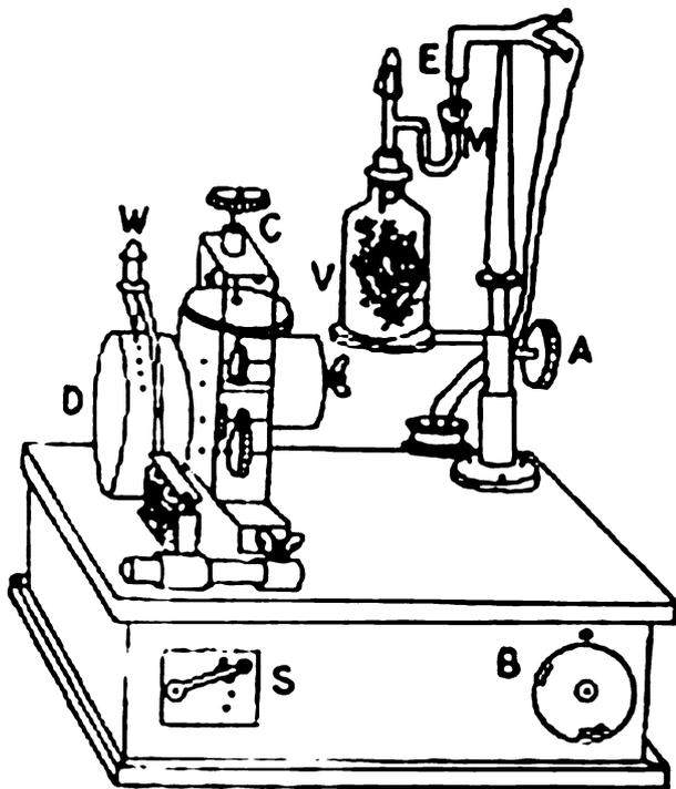
**Fig. 4** A sketch of a photosynthetic recorder of J.C. Bose. Source: S.P. Sen (1997). The symbols A, B, C, D, E, M, S, V, and W in the figure represent adjustable screw, bell, clock, drum, electrical arrangement, mercury switch, switch, glass vessel, and writing pen, respectively
