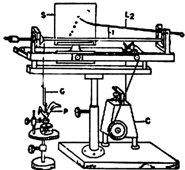
**Fig. 3** A sketch of a compound lever crescograph of J.C. Bose. *Source:* S.P. Sen (1997). The symbols C, G, L<sub>1</sub>, L<sub>2</sub>, P, and S in the figure represent clock, governor, lever 1, lever 2, plant, and screen, respectively
